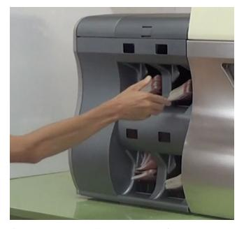
**Processing 1,000 bills a minute –** a feeder unit and a stacker unit (shown above) facilitate high-volume and high-speed processing. Banknotes are fed oneby-one from the feeder unit. Both sides are irradiated with strong UV-C light and then stored in the pocket of the stacker unit.
